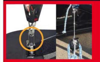
Mainsheet Ratchet Block Attachment to Hull or boom Replace the existing Wichard Snaphook with a standard quick release shackle. Careful to use quick release shackles where it is impossible to lose the quick release part. Mainsheet Ratched block attachment can be of any brand.
